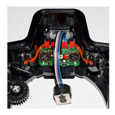
Optoelectronic TTL-Converter for CANON for SEA&SEA modern underwater housings
