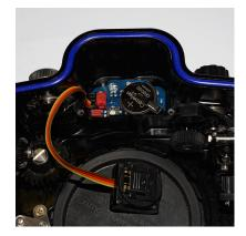
Optoelectronic TTL-Converter for SONY for SEA&SEA MDX-?U, A7II, A7III, A7IV, A1 and other underwater housings
