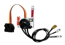
Optoelectronic TTL Converter for NIKON for ISOTTA housings, including Leak Detector system and 2 pcs LEDs (without Optical Bulkheads)
