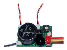
Universal Optoelectronic TTL-Converter for SONY A1-A9, including Leak Detector electronics, Sirene and Leak Sensor
