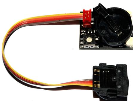
TTL-Converter for SEACAM housing for Sony A9 III camera with global shutter
