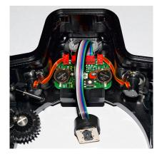
Optoelectronic TTL-Converter for NIKON for SEA&SEA modern underwater housings
