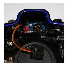
Optoelectronic TTL-Converter for SONY for SEA&SEA MDX-?U, A7II, A7III, A7IV, A1 and other underwater housings
