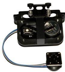
Optoelectronic TTL-Converter for SONY for MARELUX underwater housings (with metal frame)
