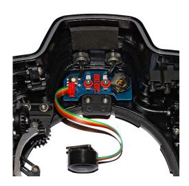
Optoelectronic TTL-Converter for CANON for NAUTICAM and HUGYFOT underwater housings
