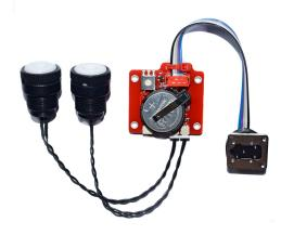
Optoelectronic TTL Converter for ISOTTA underwater housings of former years for NIKON, including 2pcs M16 Optical Bulkheads. Product 11055-HSS-M16 should be used for housings equipped with Isotta old style optical bulkheads (not separable optical bulkheads). M16 Optical Bulkheads included with the product kit should be screwed into M16 holes on the housing top.
