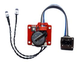
Optoelectronic TTL Converter for ISOTTA underwater housings for NIKON, including remote LEDs. Product is compatible with the housings equipped with new Isotta optical bulkheads having transparent plastic insert of standard 5mm-LED shape. Those plastic inserts should be replaced with 5mm-LEDs included with the 11055-HSS kit.
