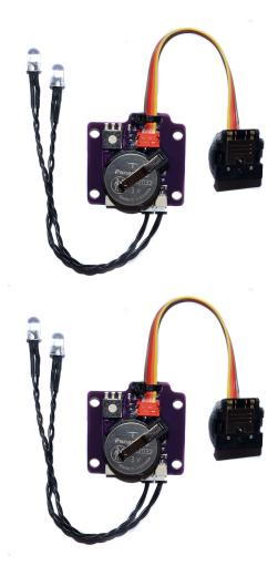
Optoelectronic TTL Converter for ISOTTA underwater housings for SONY, including remote LEDs. Product is compatible with the housings equipped with new Isotta optical bulkheads having transparent plastic insert of standard 5mm-LED shape. Those plastic inserts should be replaced with 5mm-LEDs included with the 11082-HSS kit.
