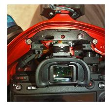
Optoelectronic TTL-Converter for SONY A1-A9 cameras for ISOTTA underwater housings, including Leak Detector system and 2 pcs Optical Bulkheads with built-in LED
