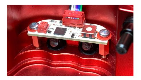
Optoelectronic TTL-Converter for OLYMPUS cameras for ISOTTA EM1-II and EM1-III underwater housings
