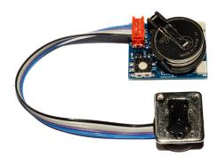
Optoelectronic TTL-Converter for NIKON for SEACAM underwater housings
