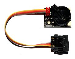
Optoelectronic TTL-Converter for SONY for SEACAM underwater housing
