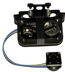
Optoelectronic TTL-Converter for NIKON Z8 for MARELUX MX-Z8 underwater housing
