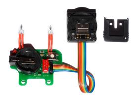
Optoelectronic TTL-Converter for SONY A7 for NAUTICAM underwater housing NA-A7
