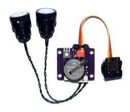
Optoelectronic TTL Converter for ISOTTA underwater housings of former years for SONY, including 2pcs M16 Optical Bulkheads. Product 11082-HSS-M16 should be used for housings equipped with Isotta old style optical bulkheads (not separable optical bulkheads). M16 Optical Bulkheads included with the product kit should be screwed into M16 holes on the housing top.
