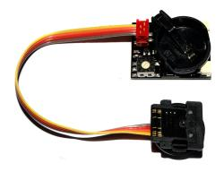
TTL-Converter for SEACAM housing for Sony A9 III camera with global shutter
