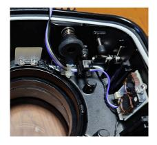
Optoelectronic TTL-Converter for SEAFROGS (MEIKON) housings for Sony A7mIV? A7rV and A7C (housings with 2 optical sockets on the top), including Optical LED module, Leak Detector system onboard
