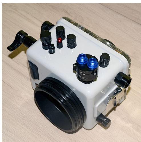
External M16-Ikelite Optical TTL-Converter for SONY A9III (camera with global shutter) for IKELITE underwater housing
