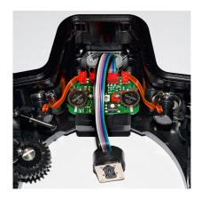
Optoelectronic TTL-Converter for NIKON for SEA&SEA modern underwater housings
